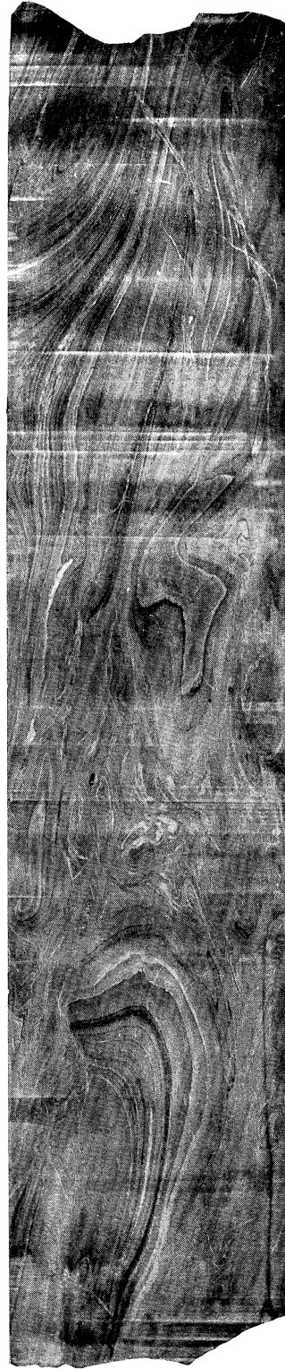
FIGURE 22. Section of a piece of core from the Weeley bore preserved in the Sedgwick Museum. This core shows remarkable structures which must have been formed while it was still plastic. The original is 4\frac{1}{2} in. wide. The transverse markings are saw cuts. The top of the core is on the left.
